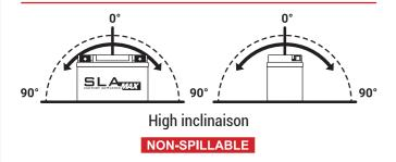
sophisticated construction design provide increased power, extended life and maximum reliability.
