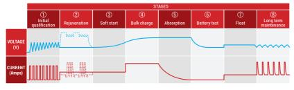
\*No float & maintenance stages for Lithium. Once the battery is fully charged, the charge is stopped.
