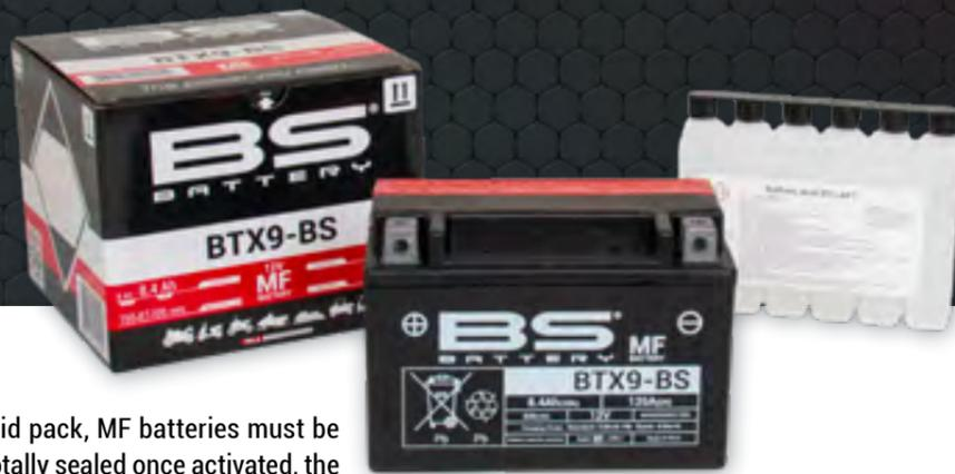
Maintenance Free batteries are designed to offer excellent power and reliability whatever the weather conditions. Supplied with an acid pack, MF batteries must be activated by filling the acid before first use. Totally sealed once activated, the gas recombination technology allows no maintenance, and does not require any water refilling. Utilizing advanced AGM (Absorbent Glass Mat) technology, these batteries are perfectly suitable for the majority of powersport applications.
