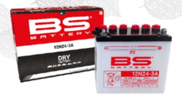
Conventional batteries are lead acid flooded batteries. These batteries need to be filled before first use. Conventional High Performance batteries include a sulfation retardant technology which reduces battery-killing plate sulfation. This results in a longer battery life, especially in standby or storage mode. These batteries are perfectly suitable for ATVs (All Terrain Vehicles), UTVs (Utility Vehicles) and lawnmowers.
